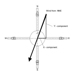
By combining the two measuring paths which are at right angles to each other, one obtains the measurement results of the sum and the angle of the wind speed vector in the form of rectangular components.
