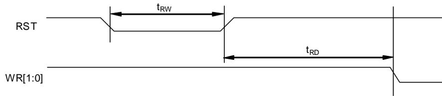
FIGURE 19: Reset Characteristics
