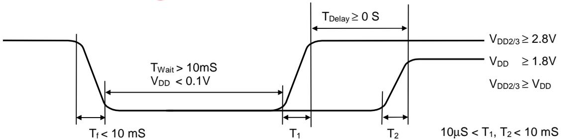
Figure 14: Delay allowance and Power Off-On Sequence
