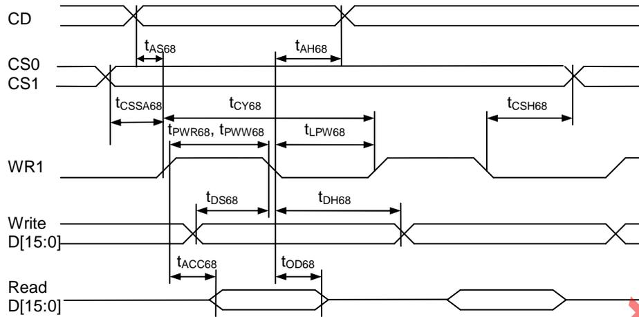
FIGURE 16: Parallel Bus Timing Characteristics (for 6800 MCU)
