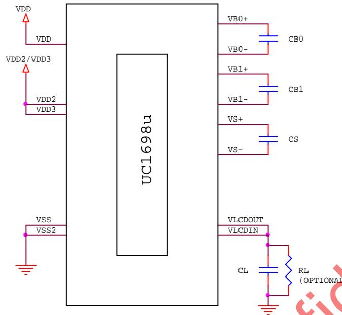
FIGURE 1: Sample circuit using internal Hi-V generator circuit
