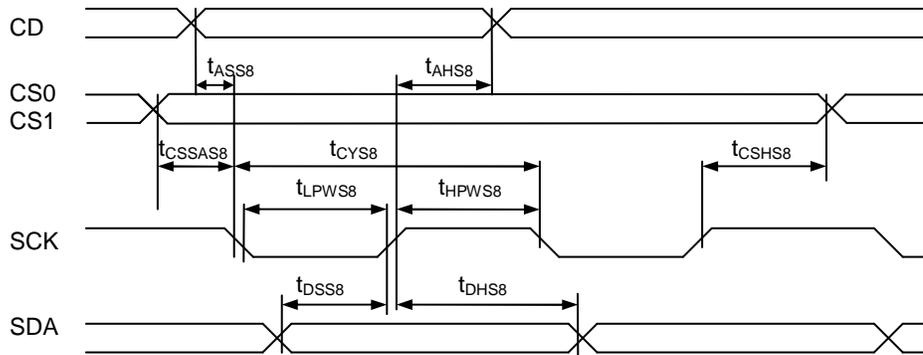
FIGURE 17: Serial Bus Timing Characteristics (for S8/S8uc)
