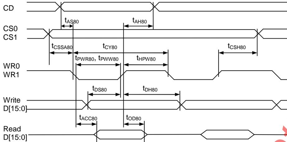
FIGURE 15: Parallel Bus Timing Characteristics (for 8080 MCU)
