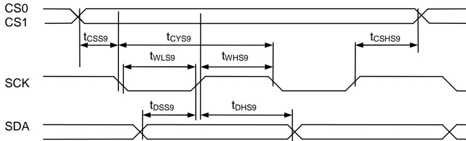
FIGURE 18: Serial Bus Timing Characteristics (for S9)
