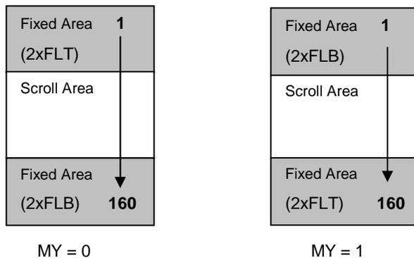
When partial display mode is activated, the display of these 2x(FLT+FLB) lines is also controlled by LC[0]. Before turning on LC[0], ensure:
