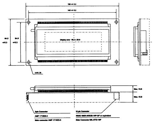
DIMENSIONS IN MILLIMETERS NOT TO SCALE, Tel +-8.5mm PCB = 1.5mm
