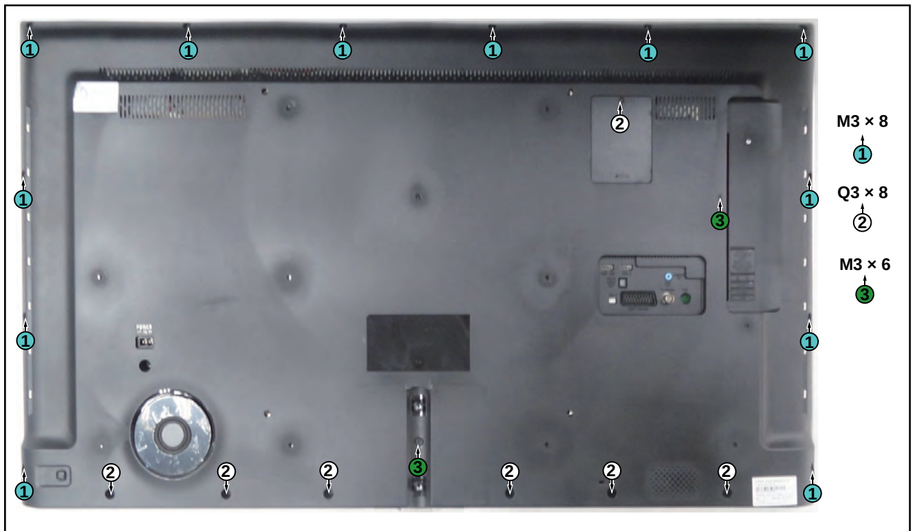
Figure 4-28 Rear cover removal[1]
