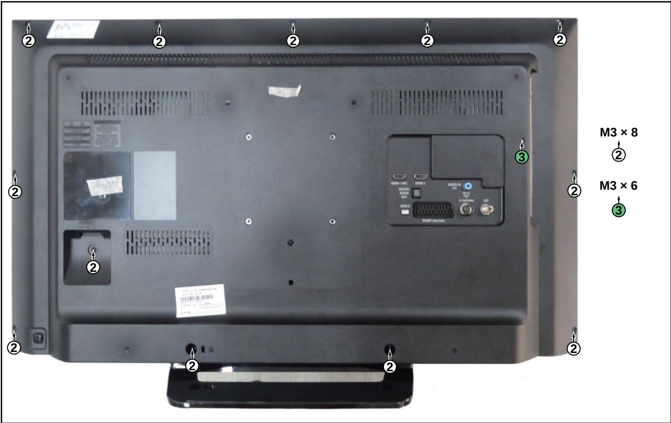
Figure 4-22 Rear cover removal
