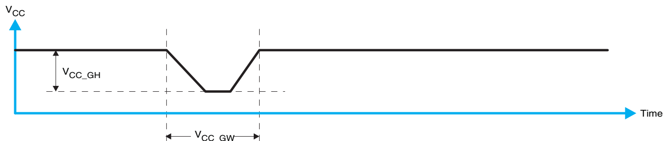
Figure 25. Glitch Width and Glitch Height
