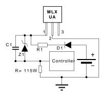
D1 Used for Reverse Voltage Protection, -24v, -150V impli Z1 Used for over voltage Protection such as +24V, 150V in R1, C1 Work with the diodes and provide conducted and ra EMC filtering.
