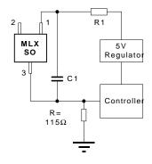
R1,C1Provide Radiated EMC filtering. Values depend on many factors. The following are suggested values.Optimum values may be determined from EMC testing. R1= $100\Omega$
