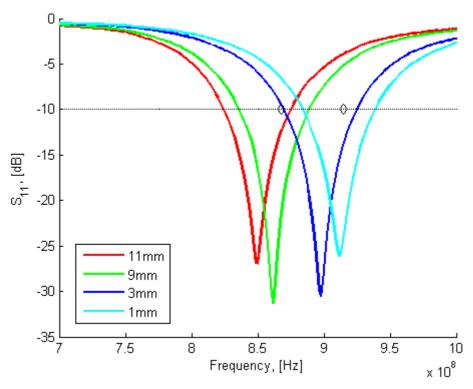
Figure 10. Measured Reflection at the End of a 15 mm long, 50  $\Omega$ , Line Feeding the Antenna. (The values in the box represent different lengths of L6.)
