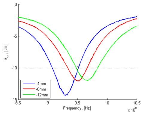
Figure 11. Measured Reflection at the Feed Point of the Antenna. (The values represent subtracted length of the antenna <u>in addition to</u> removing L6 completely.)
