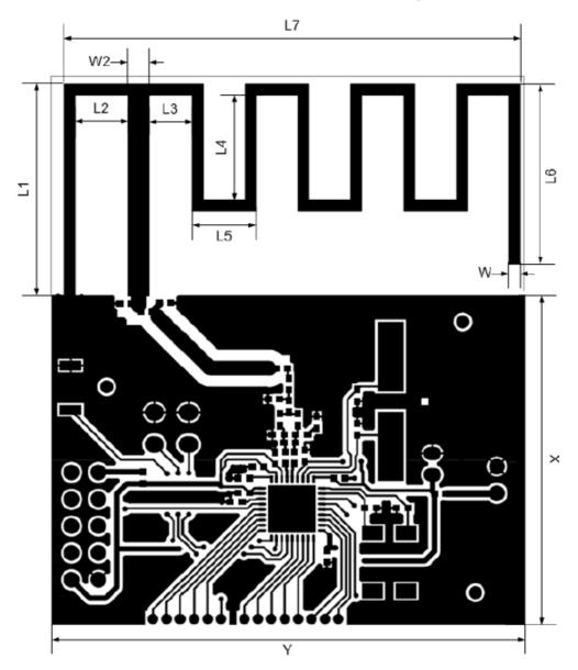
Figure 2. Antenna Dimensions
