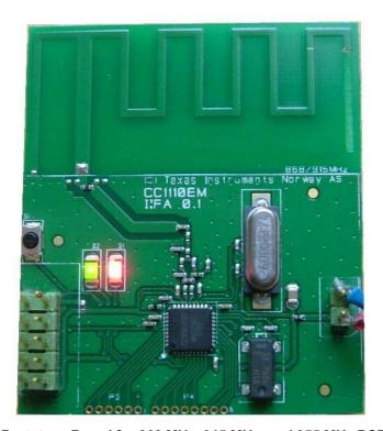
Figure 1. Prototype Board for 868 MHz, 915 MHz, and 955 MHz PCB Antenna
