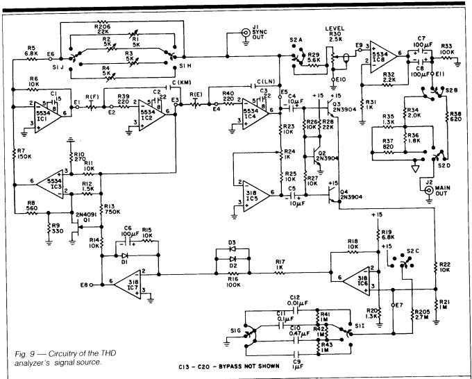
octave low-pass characteristic. Notice that the phase of this output lags that of the bandpass output by 90 degrees at all frequencies. This feature is used to provide the required 90-degree phase-shifted fundamental signal to the frequency detector in the auto-tune circuit.
