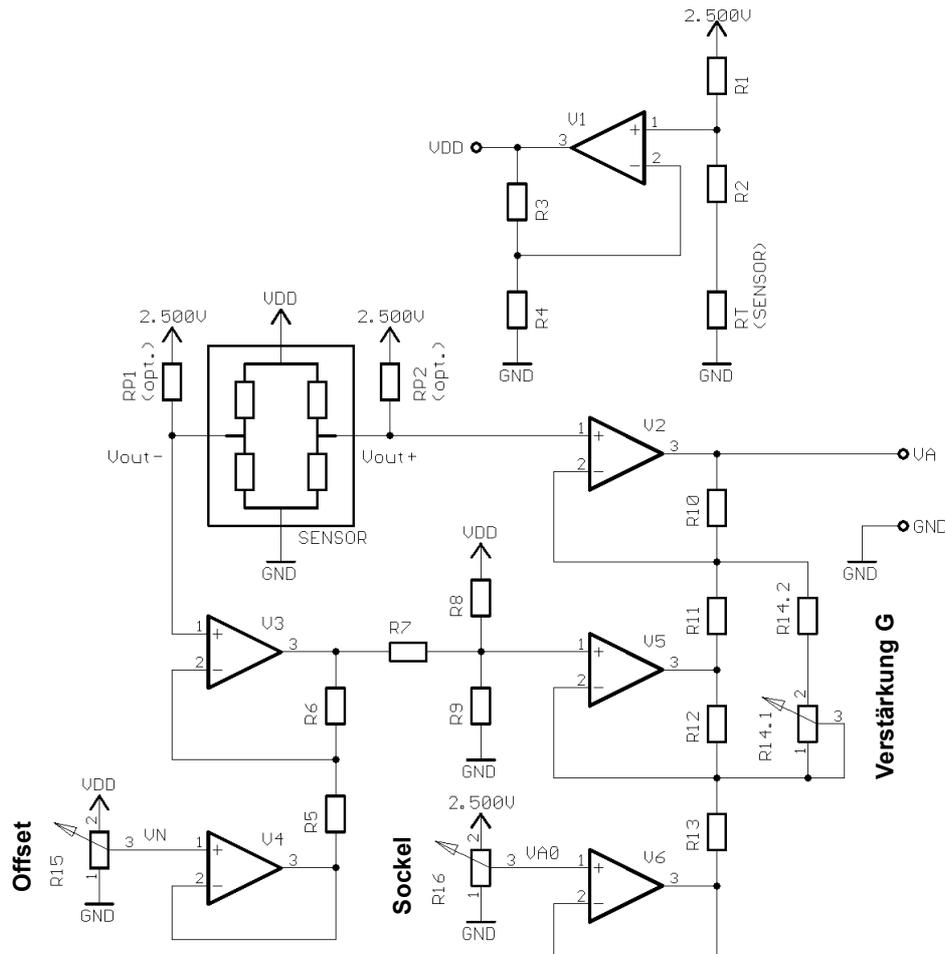
$$V_A = 2 \cdot \left(1 + \frac{R_N}{R_G}\right) \cdot \left[ (V_{out+} - V_{out-}) + \frac{R_C}{R_C + R_F} \cdot \left( V_N - \frac{1}{2} \cdot V_{DD} \right) \right] + V_{A0}$$
