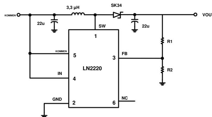
$$V_{OUT} = V_{FB} \cdot \frac{R_1}{R_2}$$
