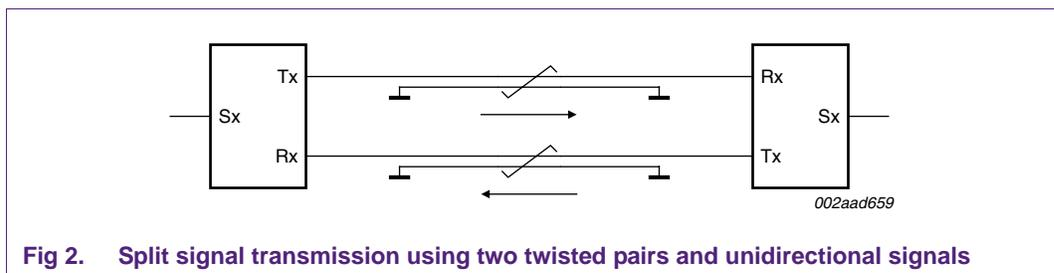
**Fig 2. Split signal transmission using two twisted pairs and unidirectional signals**
