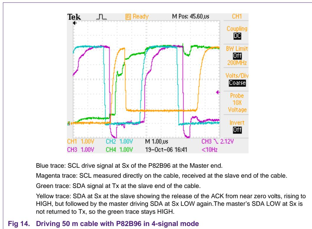
Points to note include the reasonably controlled overshoot of the falling edge of SCL at the far end of the cable to about -1 V which would still exceed the rating of Rx if the series 1 kΩ and shunt Schottky diode had not been used. The effects of cross-coupling of the 4 signals and the voltage drop on the cable resistance also results in some distortions of
