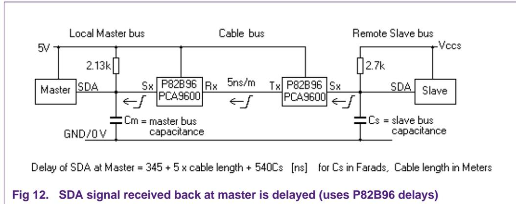
**Fig 12. SDA signal received back at master is delayed (uses P82B96 delays)**
