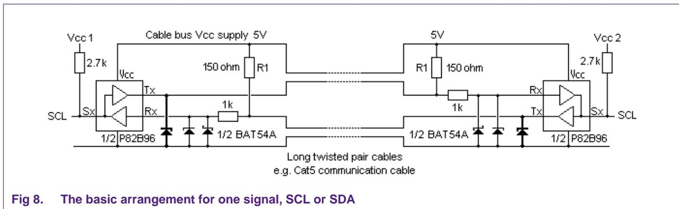
Fig 8. The basic arrangement for one signal, SCL or SDA
