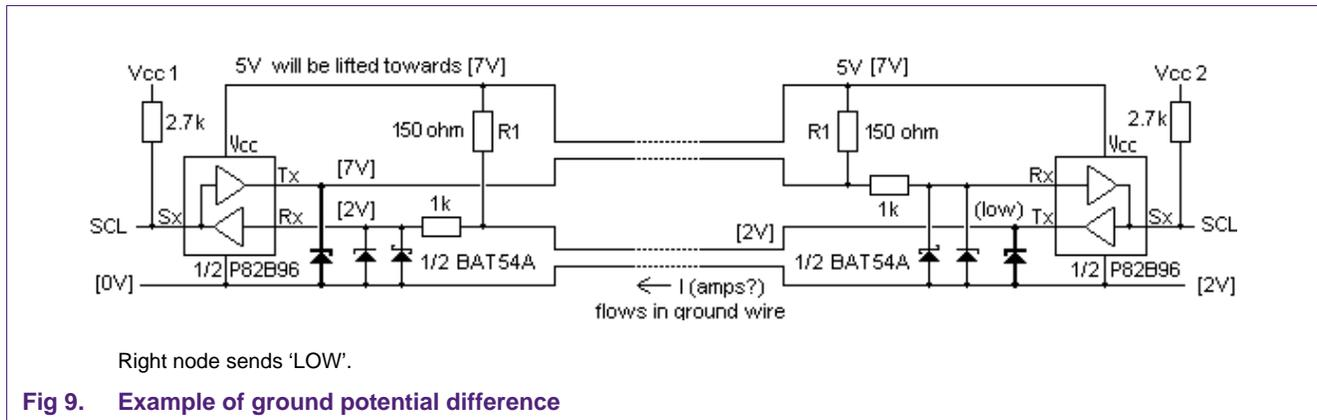
In this example it is assumed that the node on the right hand side has a ground potential that is 2 V above the ground potential of the node on the left.
