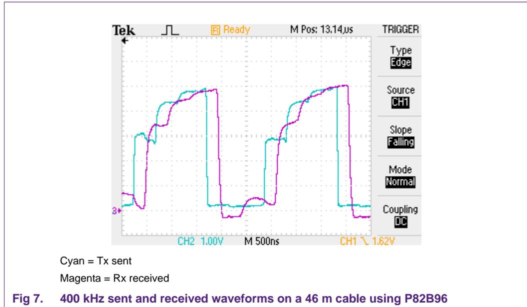
Typical waveforms on a 46 m cable are shown in [Figure 7](#). The cyan trace shows the 'send' signal generated at Tx. It is pulled LOW to approximately 0.2 V by the strong sink capability of Tx even though the 'dynamic' load is the 100  $\Omega$  cable characteristic impedance.
