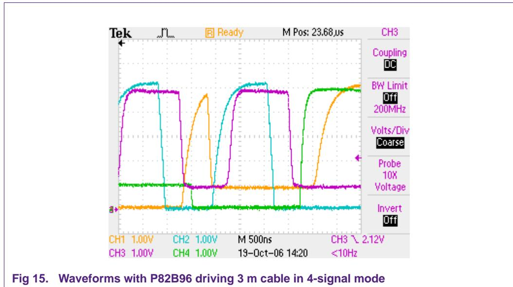
Fig 15. Waveforms with P82B96 driving 3 m cable in 4-signal mode
