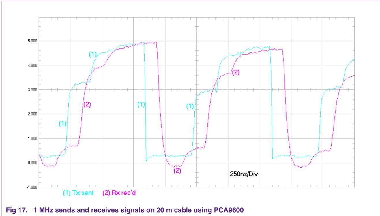
Fig 17. 1 MHz sends and receives signals on 20 m cable using PCA9600
