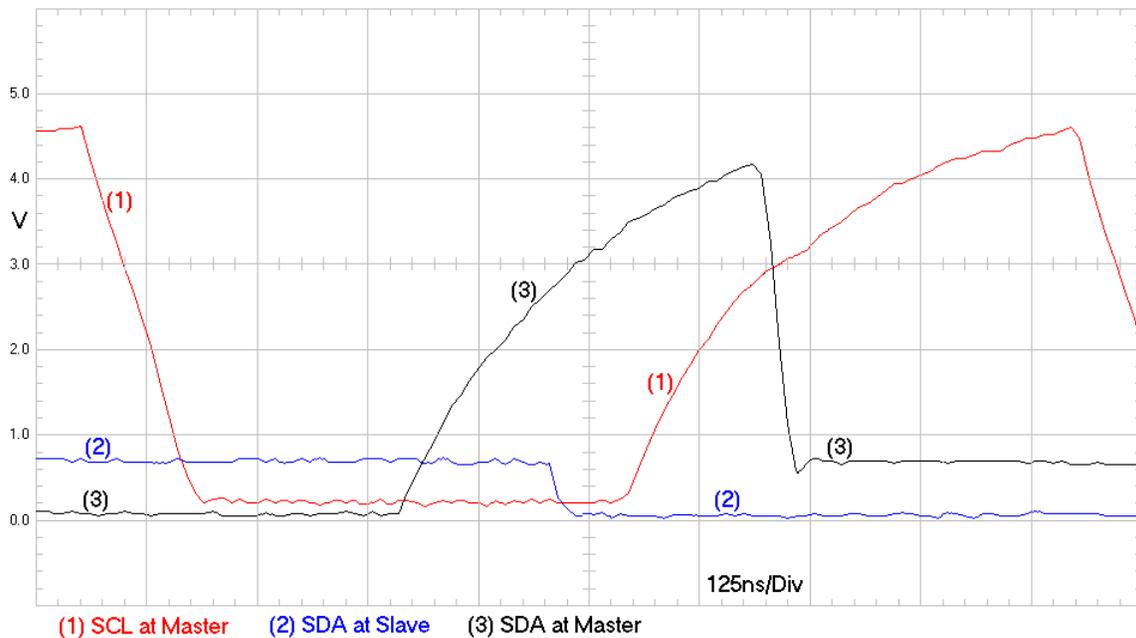
Fig 16. PCA9600 driving Fm+ slave over 20 m cable in 4-signal mode
