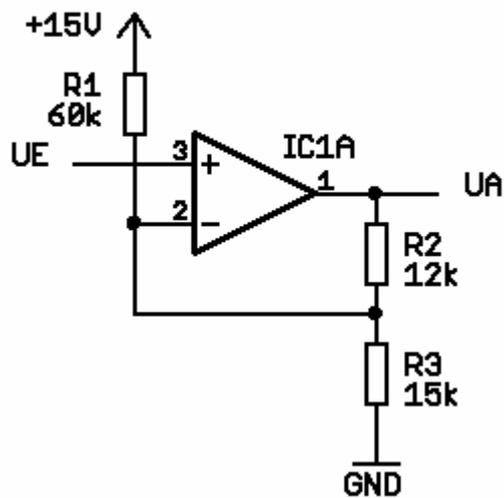
$$\frac{U_b - U_e}{R_1} + \frac{U_a - U_e}{R_2} + \frac{0 - U_e}{R_3} = 0$$
