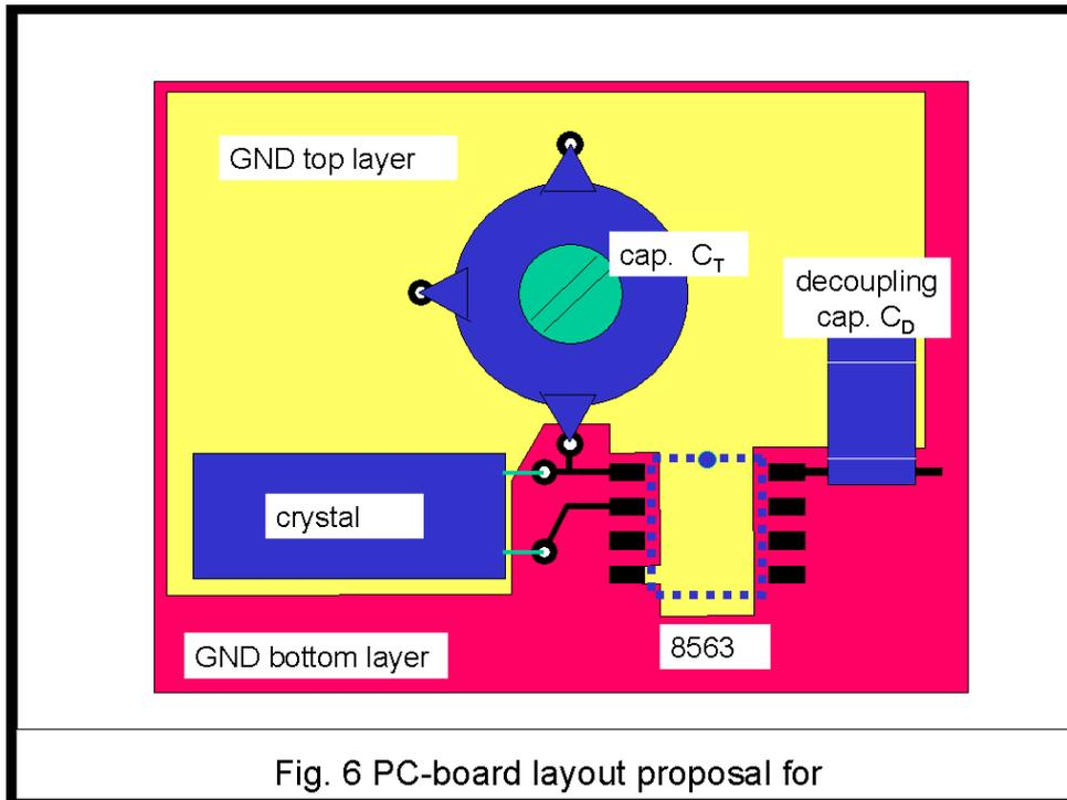
The high impedance inputs of the oscillator are sensitive to pick-up of spikes, resulting in the clock running fast. The best preventive measure is to shield the oscillator circuit and keep the connections to OSCI and OSCO at an absolute minimum. The crystal case of 8563,83,93 can be soldered to GND and for 8573 to  $V_{DD}$ .
