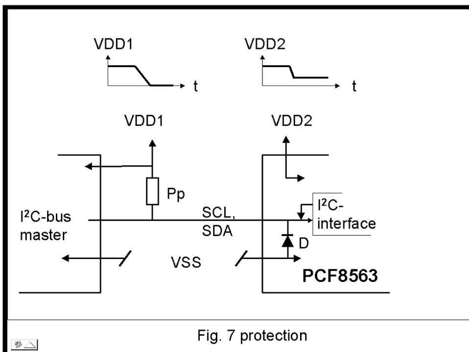
The Clock circuits PCF8563, and 8593 have on the pads SDA, SCL and INT a protection circuit with no diode to VDD. This allows to partially switch off the VDD. E.g. During operation the complete application is powered by 3.3V, then during stand-by just the RTC is operating and powered from a 0.47F-capacitor, which then will be slowly discharged to 1.5V. Check Fig 7 and 8. PCF8583 has no protection diode to VDD and the INT pin, but has diodes to VDD and the SCL, SDA pins!
