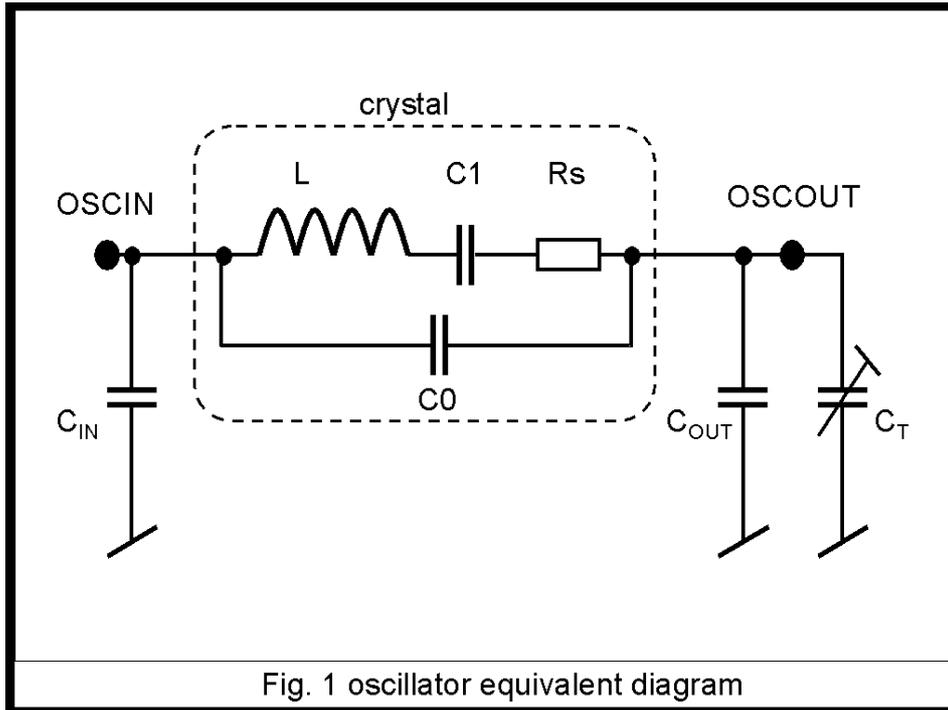
Fig. 1 oscillator equivalent diagram
