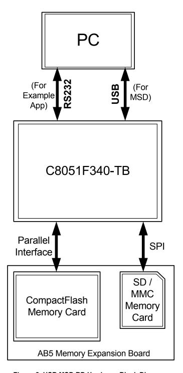
Figure 2. USB MSD RD Hardware Block Diagram
