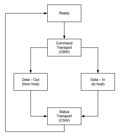
Figure 5. MSD Class - Command/Data/Status Flow
