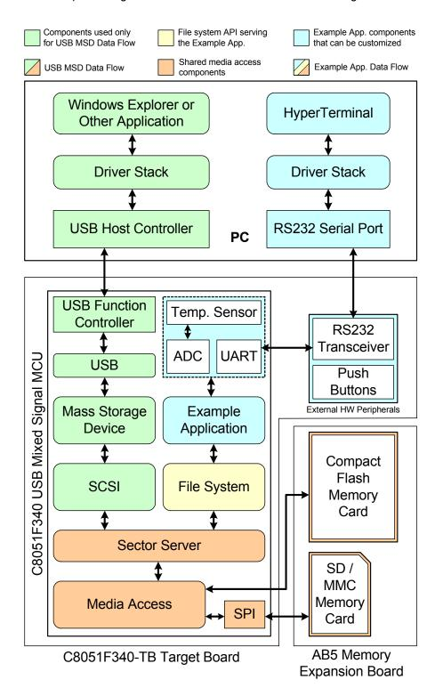
Figure 3. USB MSD RD System Architecture
