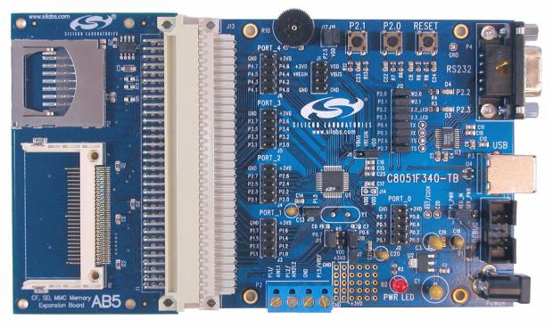
Figure 1. C8051F340-TB Target Board connected to AB5 Expansion Board
