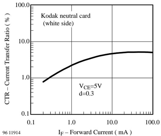
Figure 7. Current Transfer Ratio vs. Forward Current
