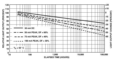
Figure 5. Projected Long Term Light Output Degradation for Pulsed Drive Conditions with the LED On-Time Duty Adjusted to Provide an  $I_{AVG}$  = 30 mA
