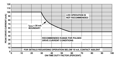
Figure 2. Recommended Range for Pulsed Drive Current Conditions for AlInGaP LEDs
