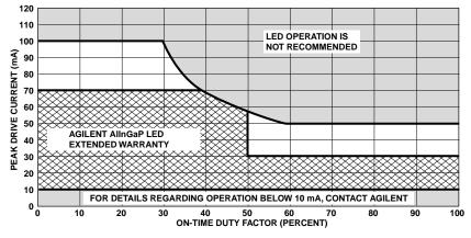
Figure 6. Agilent Technologies AlInGaP LED Extended Warranty Pulsed Current Operating Range
