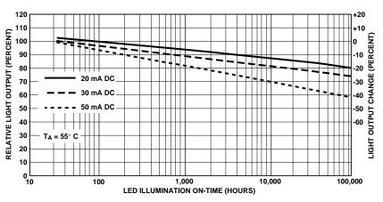
Figure 3. Projected Long Term Light Output Degradation for dc Drive Currents
