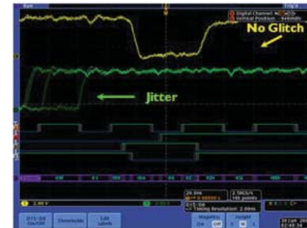
Tektronix 4000 Series update rate drops when you turn on deep memory and digital channels and the scope misses the signal jitter and metastable state
