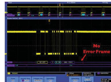
Turning on serial decoding severely limits the update rate of the Tektronix 4000 series as it is not able to capture the error frame
