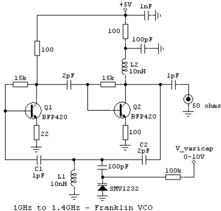
In this circuit, each stage shifts phase  $180^\circ$  so that the total phase shift is  $360^\circ$  which is equivalent to zero phase shift. We may say that one stage serves as the phase inverting element in place of the RC or LC network which generally performs this function. It is, from an analytical viewpoint, immaterial which stage we choose to look upon as amplifier or phase inverter.
