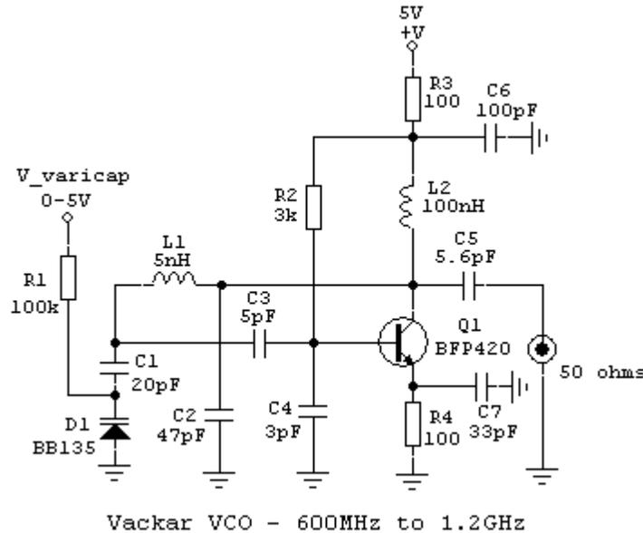
The Vackar VCO circuit incorporates a  $\pi$ -section tank to attain the needed  $180^\circ$  phase-reversal in the feedback loop.
