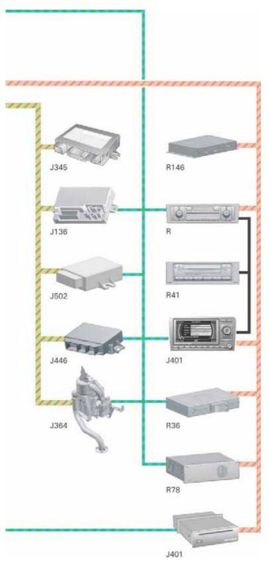
The bus topology - as with the complete electrical system - is heavily based on the Audi A4 '01. As before, the gateway is integrated in dash panel insert J285. To diagnose on the driveline CAN bus the control units adopted from the Audi A3 and Audi A6, the driveline CAN bus is connected directly to the diagnosis plug. The control units on the convenience CAN bus and on the infotainment CAN bus are also diagnosed via the K and L wires (see also chapter "Diagnosis", page 10).
