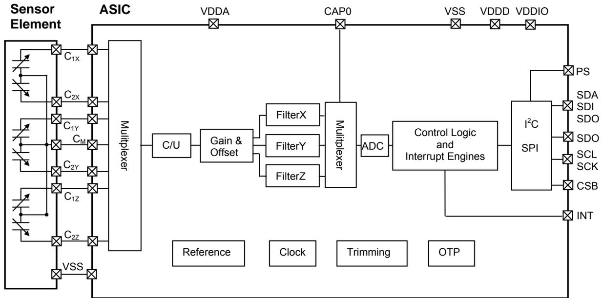
Figure 1: Block diagram BMA220
