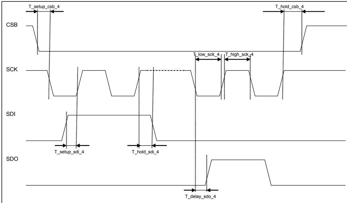
Figure 17: Timing diagram of 4-wire SPI cycle
