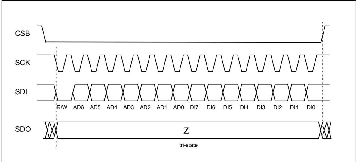
Figure 15: 4-wire SPI write command
