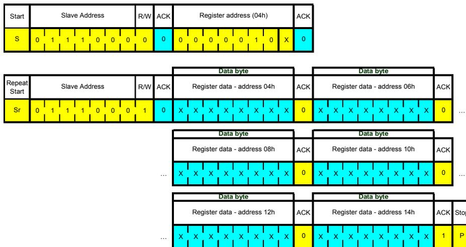
Figure 23: I<sup>2</sup>C multiple bytes read protocol
