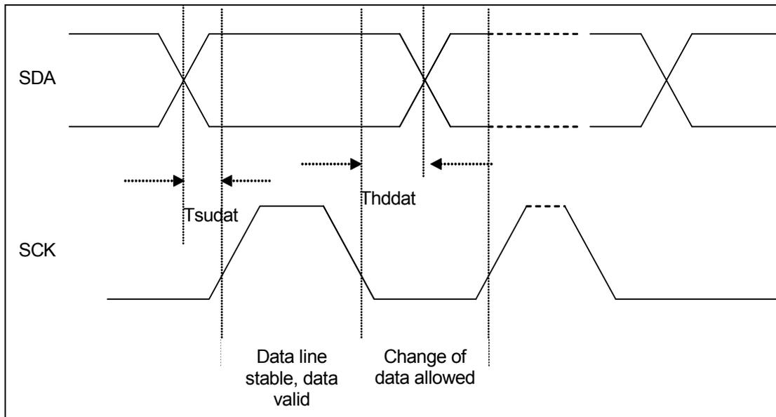
Figure 21: Waveform diagram for one bit transfer with I<sup>2</sup>C interface
