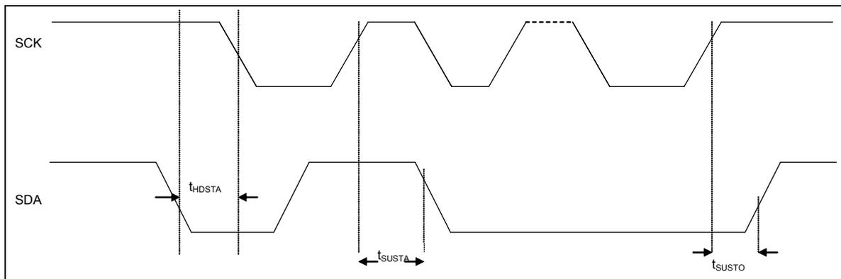
Figure 19: Waveform diagram for I<sup>2</sup>C start and stop conditions
