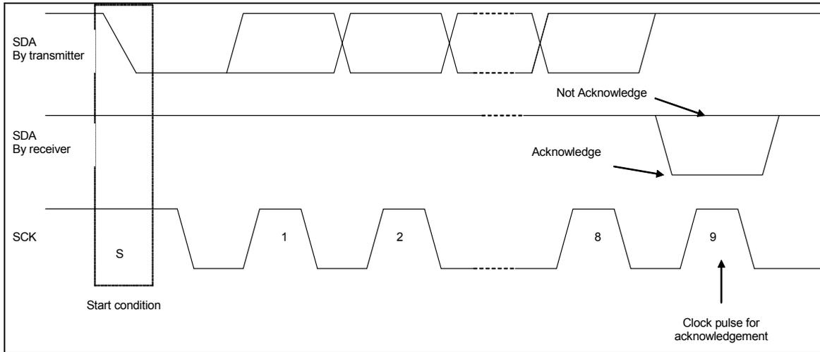
Figure 20: Waveform diagram for I<sup>2</sup>C acknowledgement on SDA
