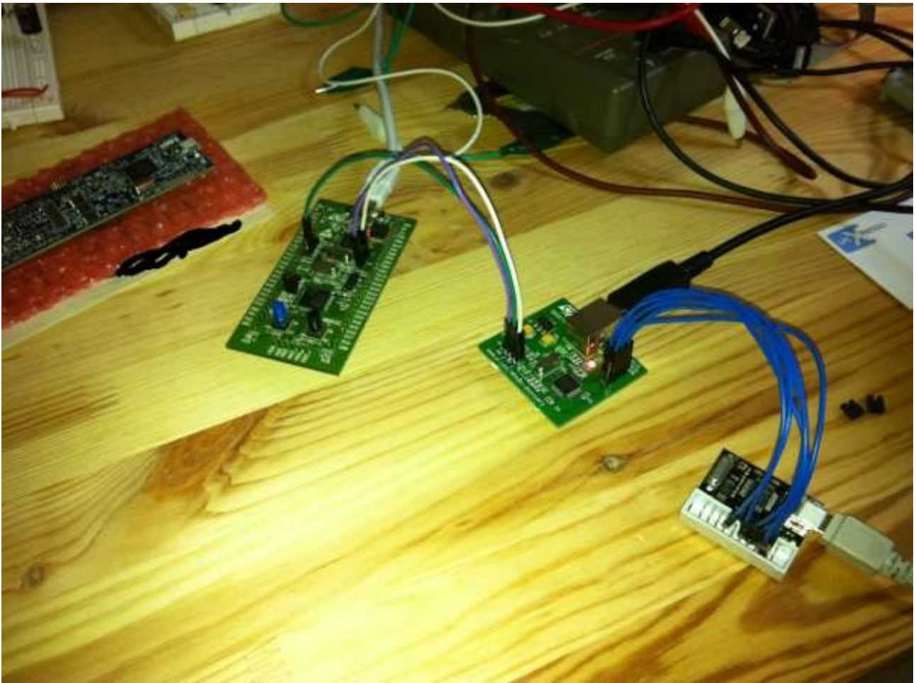
The complete STM8S conversion/test setup
