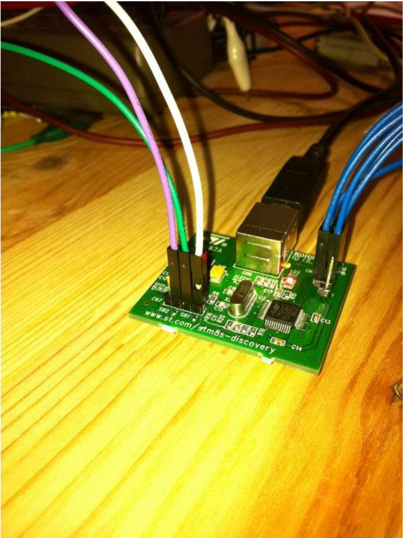
The finished STM8S SWD debugger Blue wires on JTAG , and SWDwires on CN7 Purple = SWDIO - Green = GND – White= SWCLK
