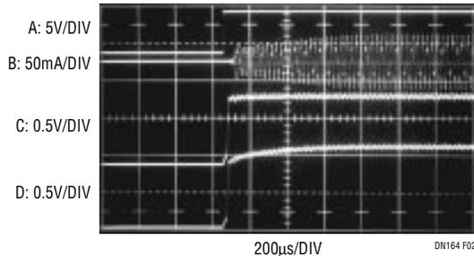
**Figure 2. Fast Loop Response Maintains Regulation at 200Hz PWM Rate. Waveforms Include PWM Command (A), Lamp Current (B), LT1371 Feedback (C) and Error Amplifier  $V_C$  (D) Pins. Loop Settling Occurs in 500µs**
