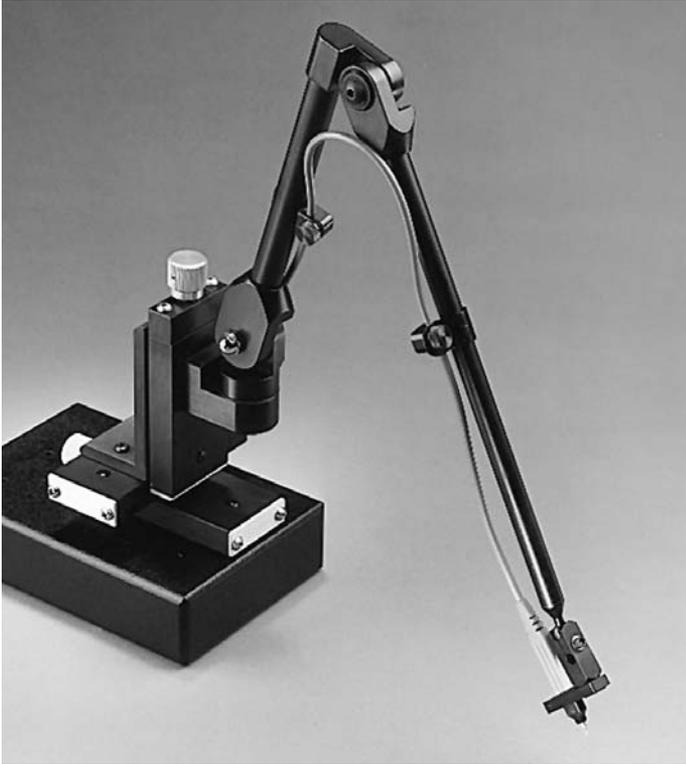
**Figure 2.10.** Example of a probing station designed for probing small geometry devices such as hybrid circuits and ICs.
