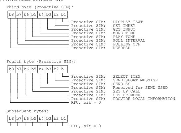
RFU bits, and all bits of subsequent bytes, are reserved to indicate future facilities. A SIM supporting only the features of SIM Application Toolkit defined here shall not check the value of RFU bits.
